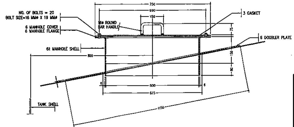
ROOF MANHOLE SECTION
