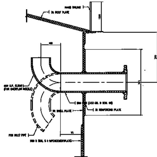
INLET/OVERFLOW NOZZLES (TYPICAL)
