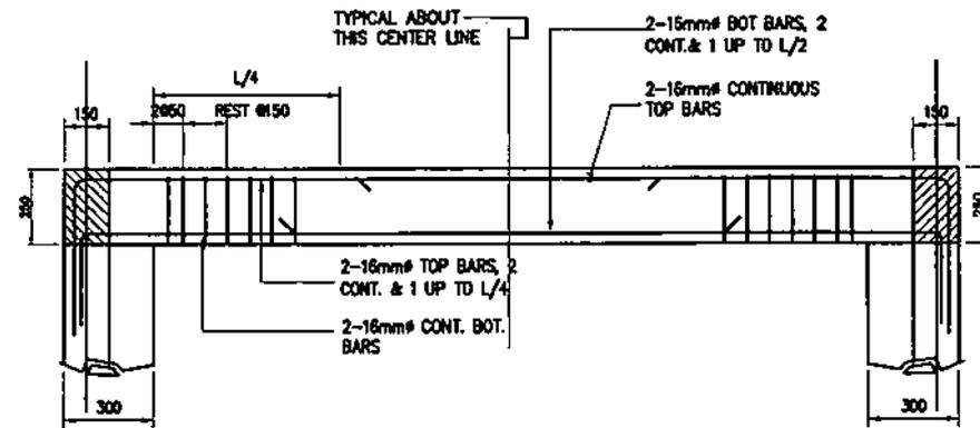
**ROOF SLAB REINFORCEMENT**
