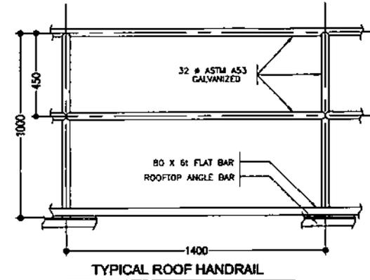
**TYPICAL ROOF HANDRAIL**
