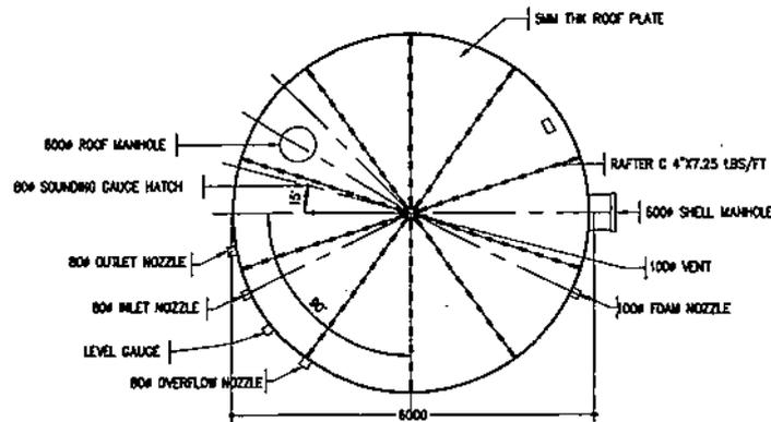
ROOF PLATE ARRANGEMENT & NOZZLE ORIENTATION
